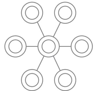
With distributed split, a single fiber between the terminal and splice case is used, and the terminal incorporates a 1x4 or 1x8 splitter. Distributed split architectures use about the same amount of cable as centralized, but the fiber counts are a fraction, as are, consequently, the splicing costs.
