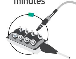
Use of pre-terminated connectors eliminates splicing, thus reducing the total time of connecting a customer to the fiber network
