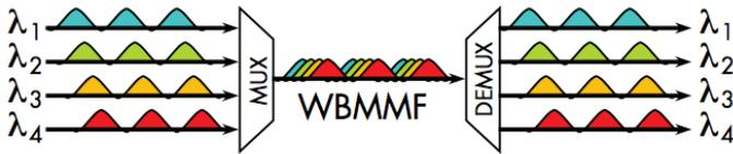
Figure 5 - WDM concept showing four wavelengths
