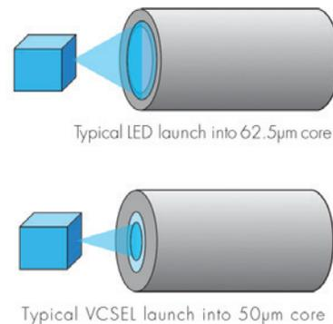
Figure 1 - Overfilling LED and under-filling VCSEL launches
