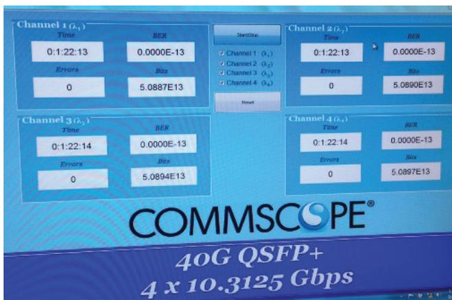
Figure 10 - 40G-SWDM4 over 500 m of LazrSPEED 550 WideBand MMF at BICSI
