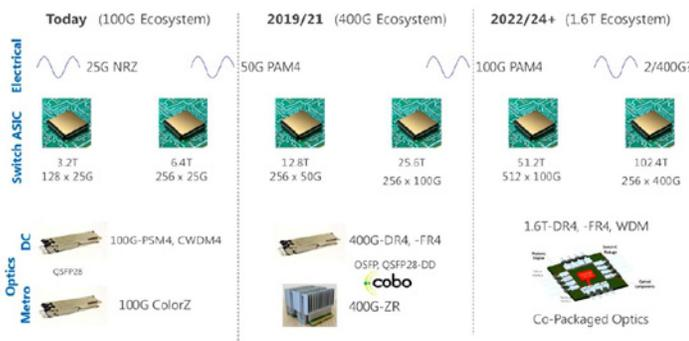
Figure 1: Chip I/O and optical integration
