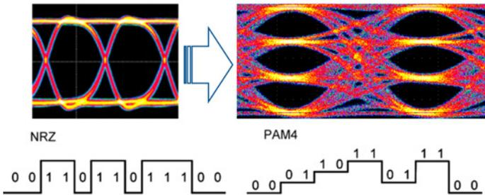
Figure 9: PAM4 modulation versus NRZ
