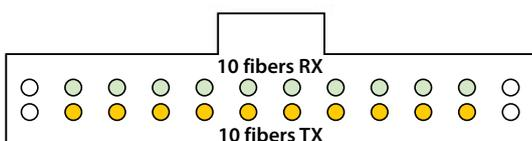
Figure 5: MPO connector pinout for 100GBASE-SR10
