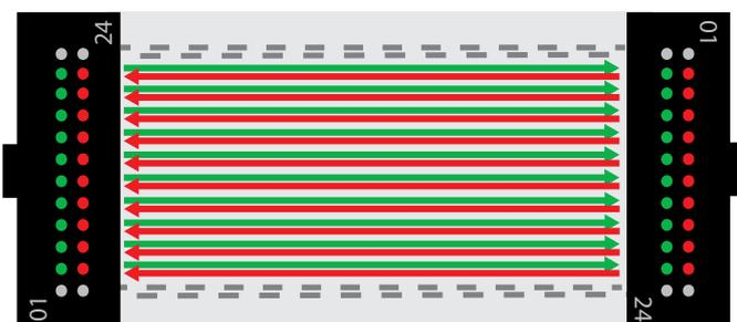
Figure 4: 100GBASE-SR10 full duplex operation on 20 fibers
