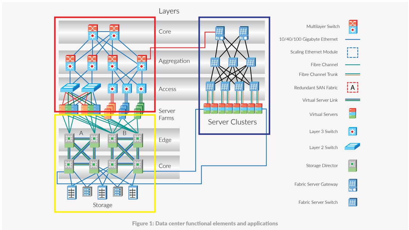
Figure 1: Data center functional elements and applications
