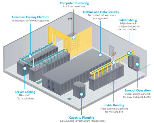
Figure 8: Cabling system infrastructure
