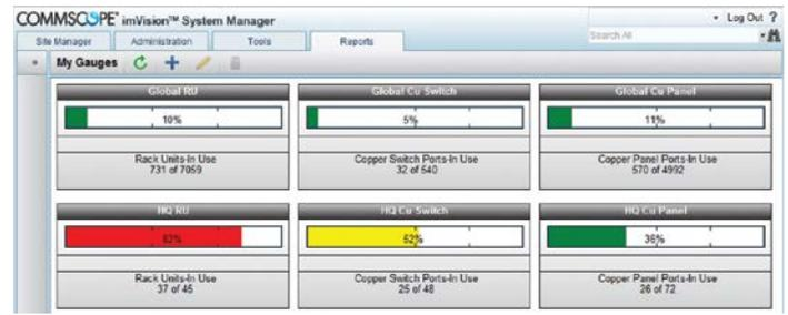
A capacity management dashboard from CommScope's imVision® AIM solution
