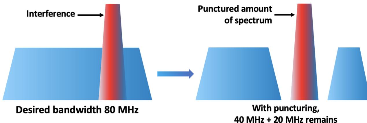
Figure 3: Punctured Transmission on a Channel
