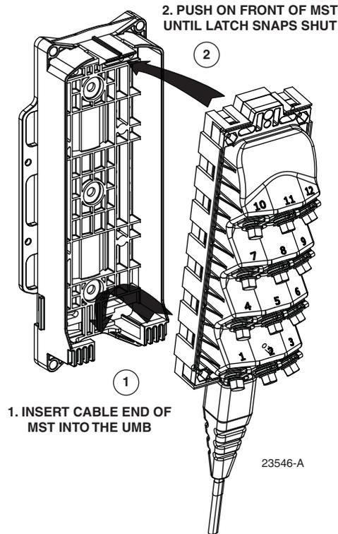
Figure 11. Installing the MST in the Universal Mounting Bracket
