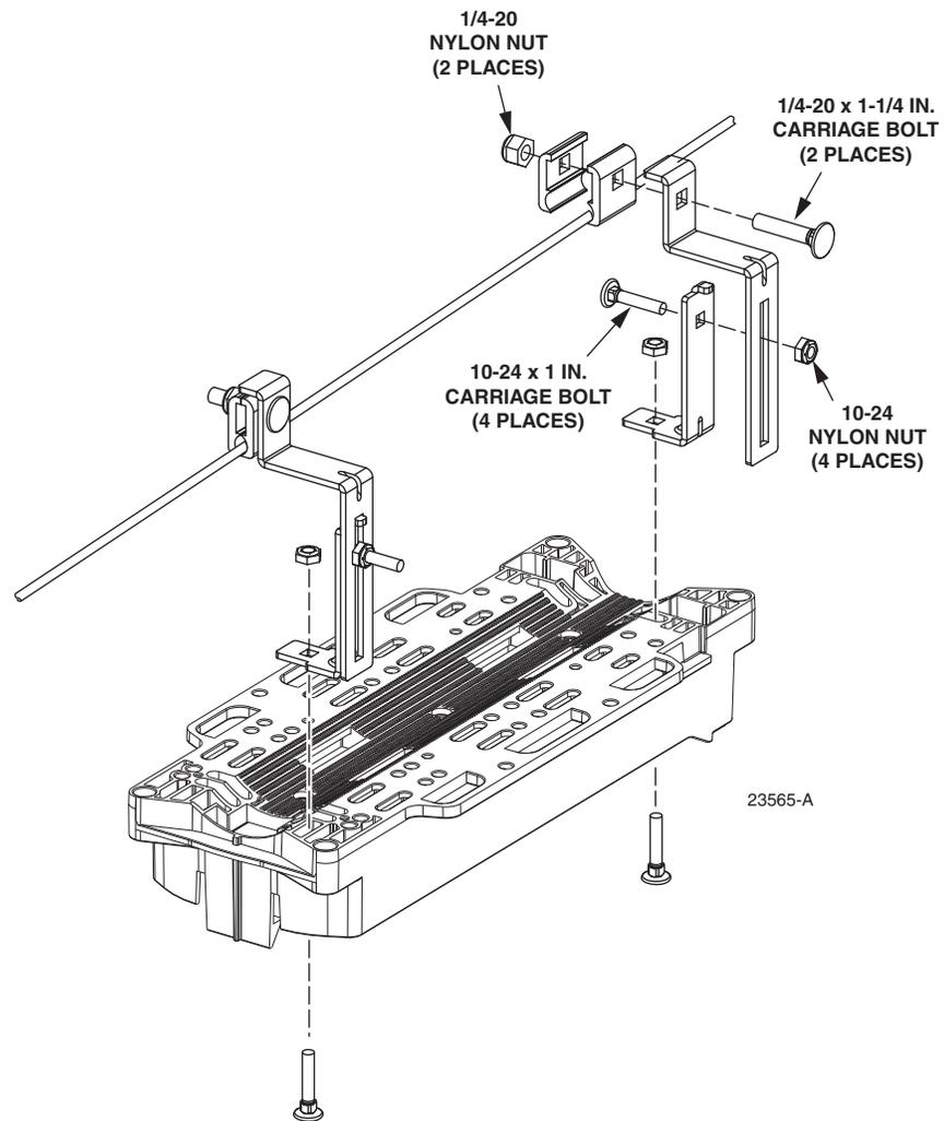
Figure 12. Securing Strand-Mounted MST
