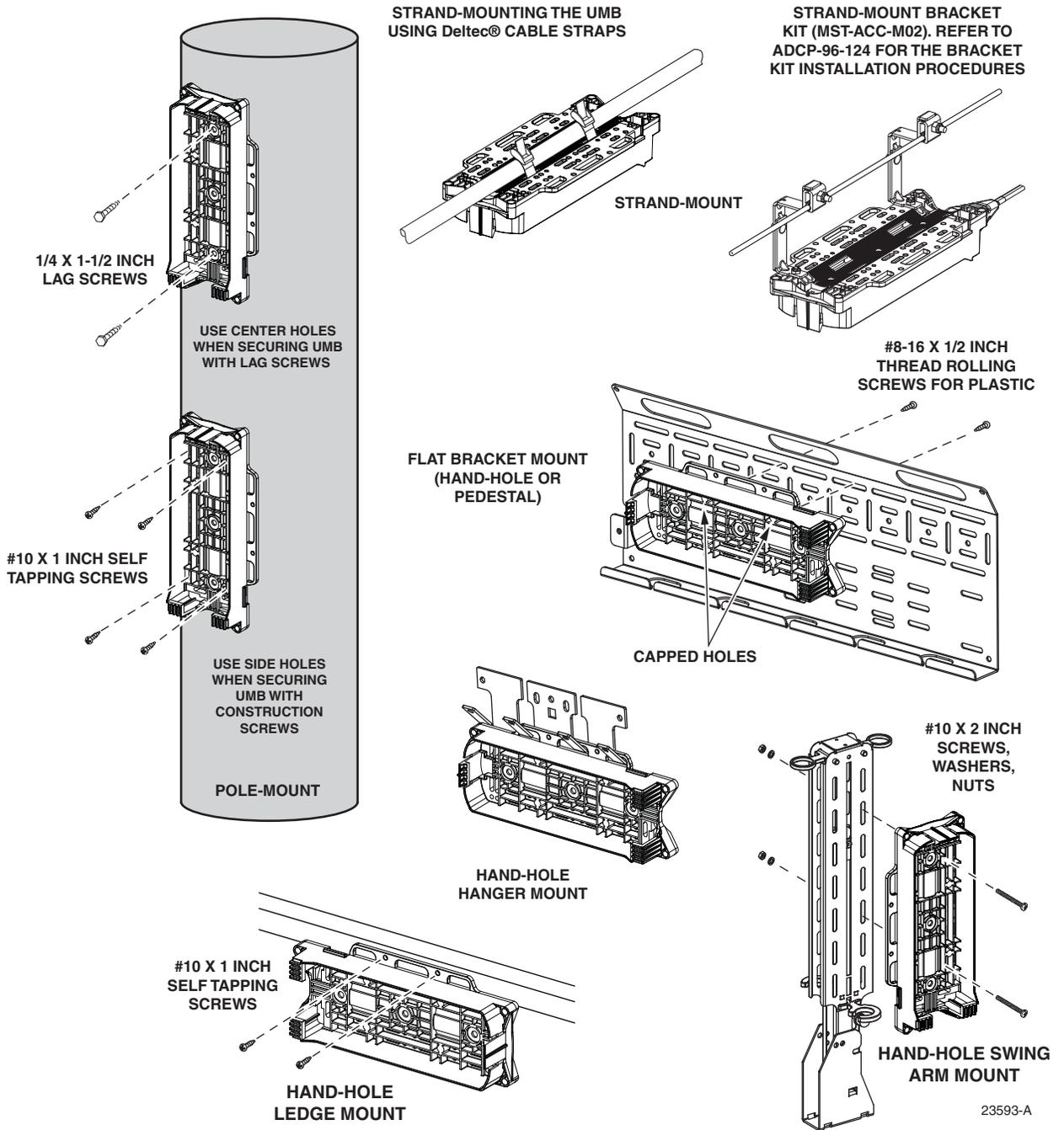
Figure 10. Typical Installation of a Universal Mounting Bracket (UMB)
