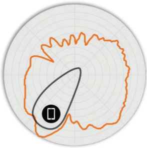
Figure 6. T670 5GHz Elevation Antenna Patterns
