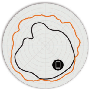
Figure 3. T670 5GHz Azimuth Antenna Patterns
