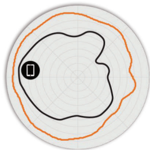
Figure 2. T670 2.4GHz Azimuth Antenna Patterns
