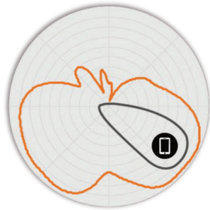
Figure 5. T670 2.4GHz Elevation Antenna Patterns
