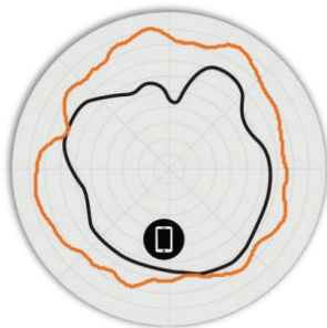
Figure 4. T670 6GHz Azimuth Antenna Patterns
