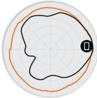
Figure 3. 5GHz Azimuth Antenna Patterns
