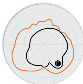
Figure 3. R350 5GHz Azimuth Antenna Patterns
