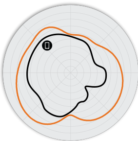
Figure 2. R350 2.4GHz Azimuth Antenna Patterns
