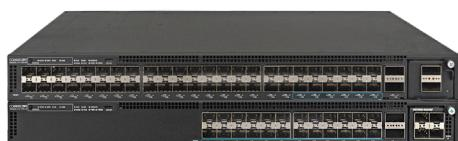
The RUCKUS ICX 7550 fiber models come in 24- and 48-port versions with a mix of 1G and 10G SFP/SFP+ ports offering class leading port density as an entry level 10G aggregation solution
