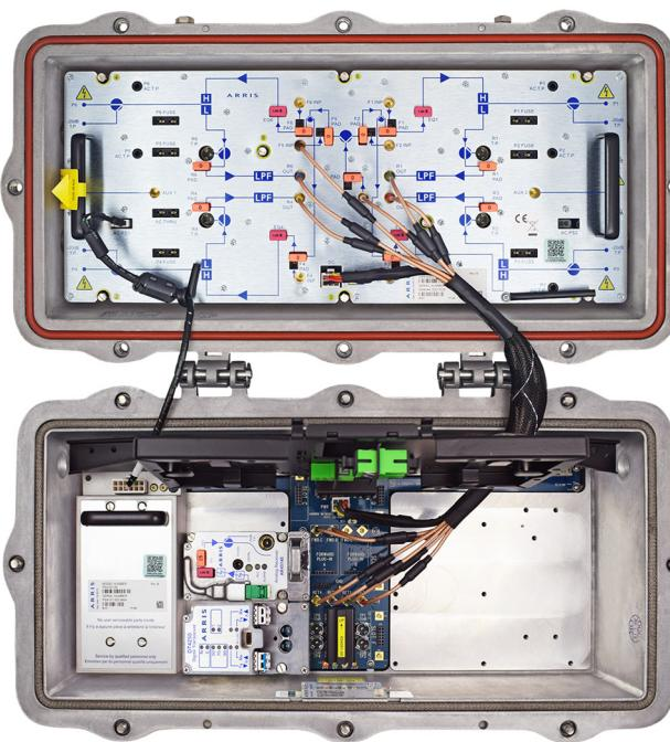
With a wide selection of customized optical passives, field-hardened EDFAs, and optical switches the node platform can extend the deployment of advanced, high-availability, “bandwidth-hungry” services into fiber-poor areas while reducing real estate and powering requirements in the field. Remote monitoring is provided via an integrated network management plug-in eliminating the added cost of a third-party status monitoring transponder system.
