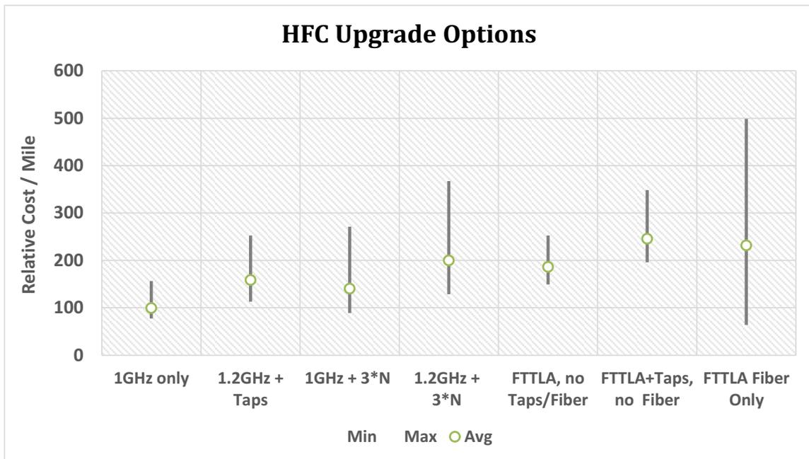
Figure 12 – Relative Cost per Mile for Various HFC Upgrade Options
