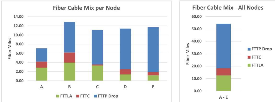
Figure 14 – Fiber Cable Mix: FTTLA, FTTC, FTTP
