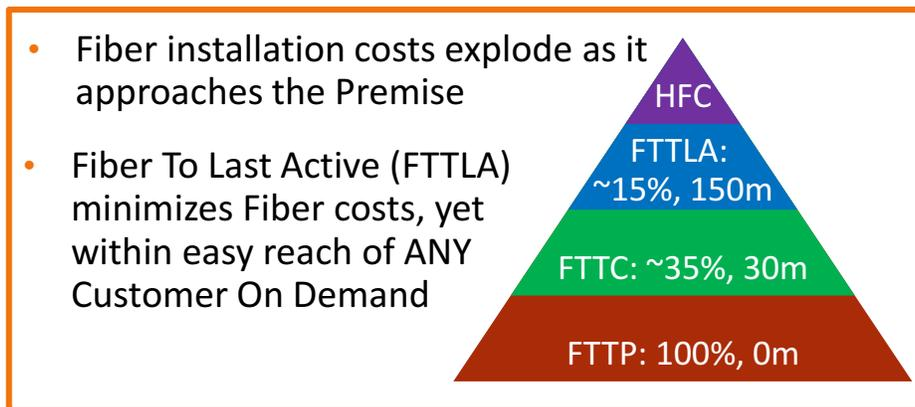
Figure 15 – Fiber Cable Mix: FTTLA, FTTC, FTTP
