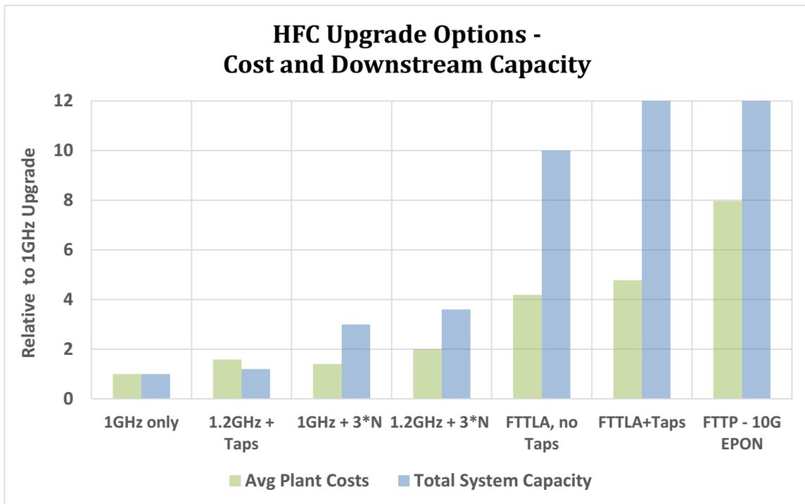
Figure 13 – Relative Cost and Capacity for Various HFC Upgrade Options
