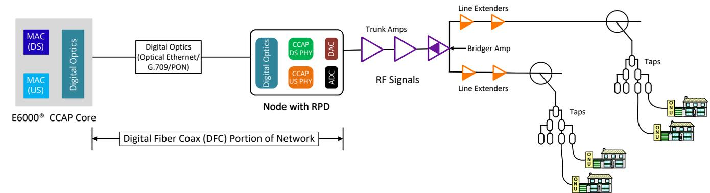
Figure 2. DAA Network Architecture with an R-PHY Node
