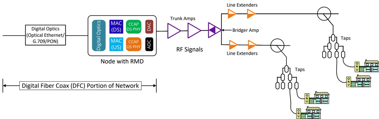
Figure 3. DAA Network Architecture with an R-MACPHY Node
