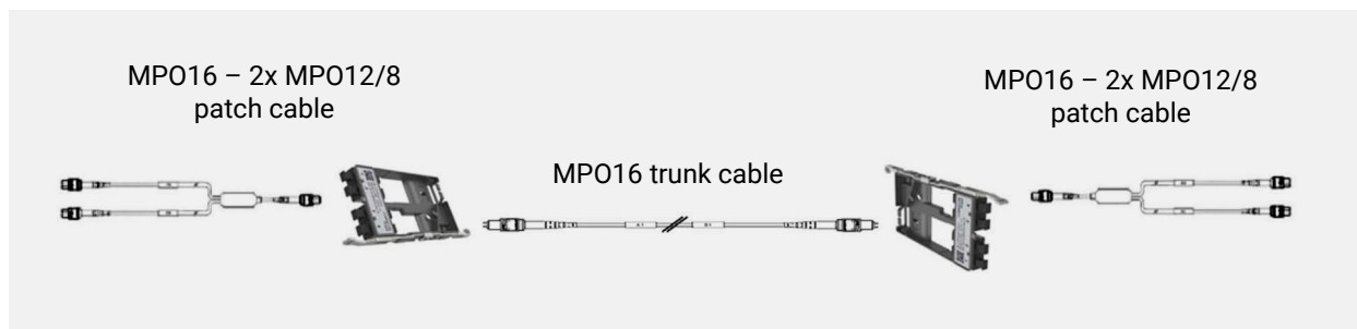
Figure 2. SCS channel using MPO trunk through adapters to breakout cables
