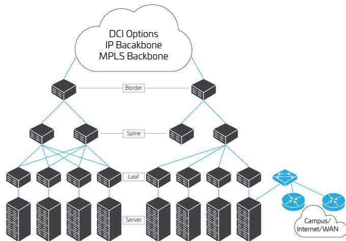
Figure 2: Placement of border-edge switches
