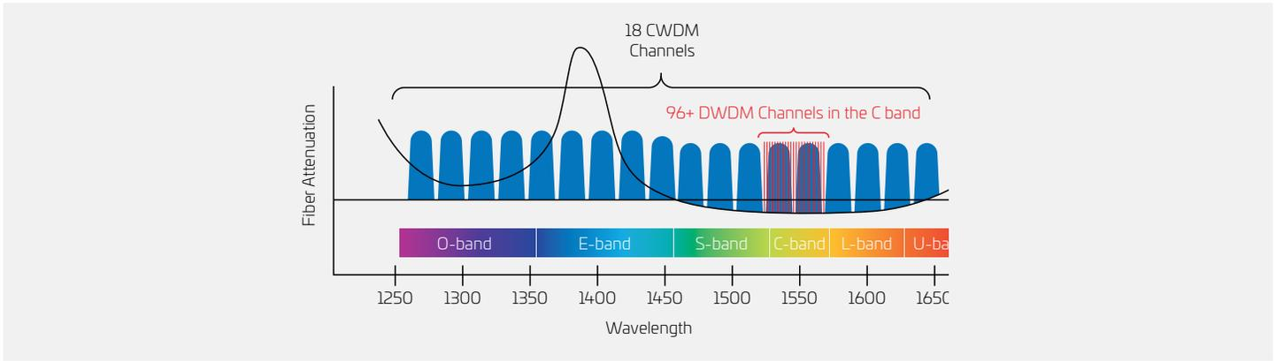
Figure 5: CWDM/DWDM band and channel configurations
