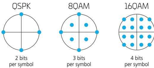
$$\text{Transmit bit rate} = [\text{symbol rate}] \times [\text{bits per symbol}] \times [\text{polarization} (x2)]$$
