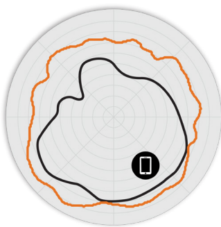
Figure 3. R770 5GHz Azimuth Antenna Patterns
