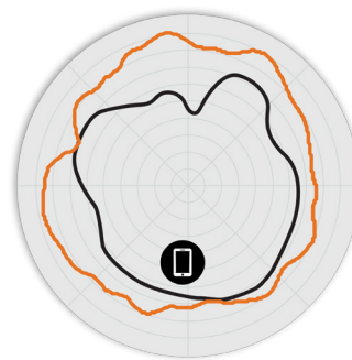
Figure 4. R770 6GHz Azimuth Antenna Patterns
