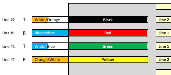
RJ-11 Hook Down Diagram ©SCTE
