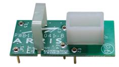
The CE-120-\* Series are used to plug into the Carrier Board for Forward Balancing and have a 1.2" height. The maximum height for any plug-in equalizer, cable simulator, and PAD inserted in the carrier board is 1.2 inches. Using plug-in accessories that exceed 1.2 inches in height will cause interference when the housing is closed and may cause damage or compromise performance.
